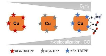
Schematic representation of the proposed mechanism for ethylene ( $C_2H_4$ ) promotion in  $Cu_{cub}$ /Fe-Por tandem catalysts.
